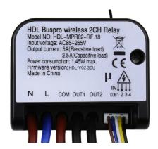
HDL-MPR02-RF.18 Buspro wireless 2CH relay, has 4CH dry contact, can control target by switch. This module should work in conjunction with wireless gateway.
