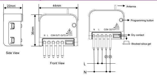
Programming button: When it is working properly, the green light will flicker, press the button three times continuously, the green light will flicker quickly, enter the setup mode. (the gateway should enter the setup mode at the same time, and then, set the parameter)
